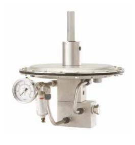
The Mark 695 Series piloted soft seat regulator is designed specifically to provide accurate pressure control on very low pressure trank blanketing systems. The pilot operated Mark 695 responds to very small changes in tank pressure by throttling open or closed to maintain the desired pressure set point.
